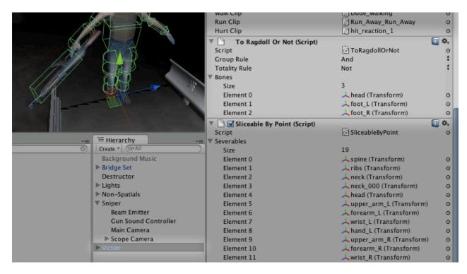
This component is called upon during the slice. It checks for the **presence** of bones in any given slice result. In the demo, we list the head, foot\_L and foot\_R bones by adding their transforms to the Bones list.
